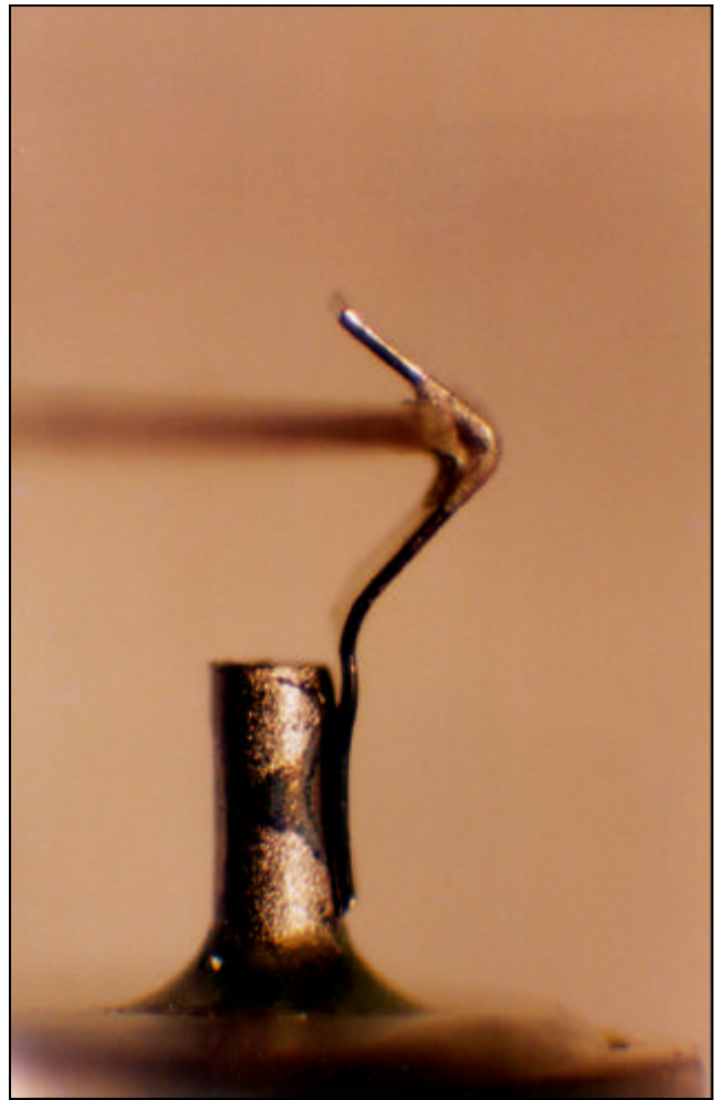
Figure 5: Photograph of side view showing insufficient adhesive.
