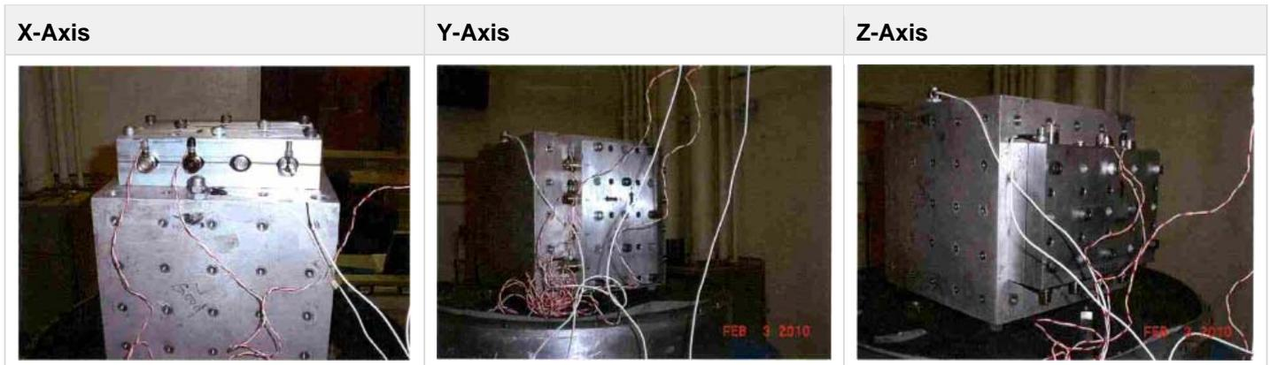
Table 2 shows pictures of a heated Random Vibration test setup. This particular heated test used flexible heaters with backing plates. The Y-Axis in this test was done with by rotating the transducers in the fixture.
