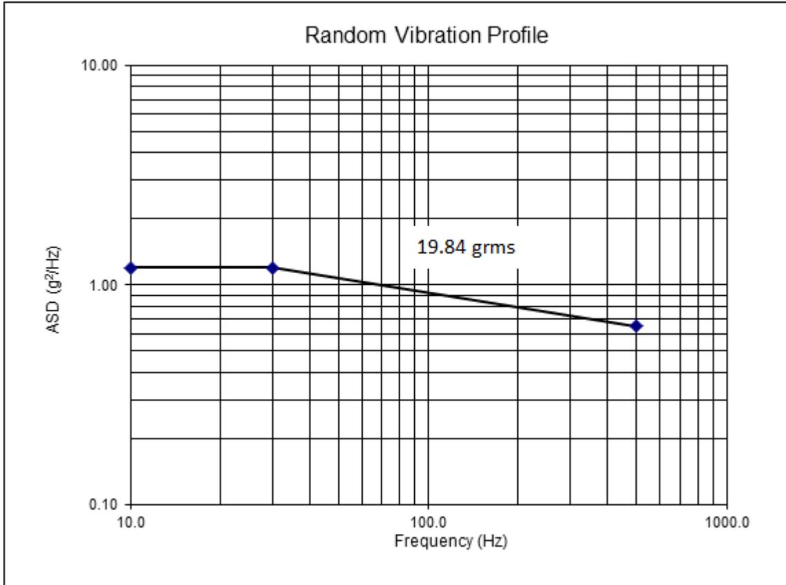
Figure 2. Typical 500 Hz Random Vibration Profile
