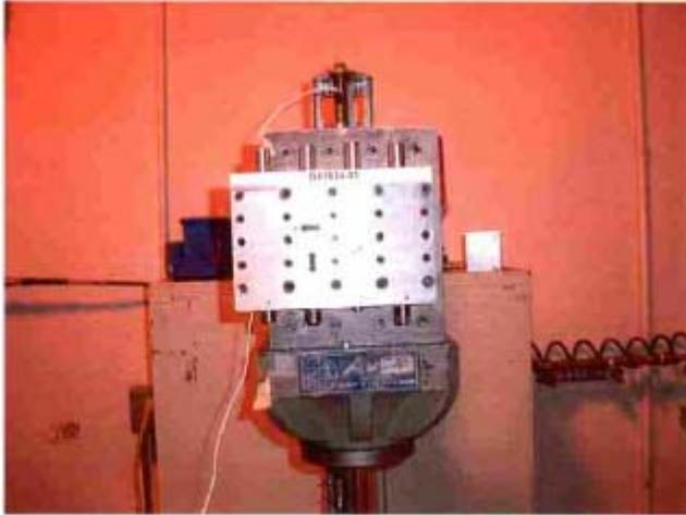
Figure 5. Quartzdyne Transducers Mounted on Drop Shock Machine for 500 g Shock Test
