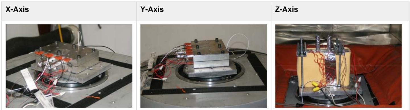
Quartzdyne has found cartridge heaters inserted into the fixture to be very effective and robust. Figure 4 shows a Random Vibe test of large electrical components with differing attach methods. The fixture is outfitted with two cartridge heaters and a cartridge style thermocouple for control. The vibration level was upwards of 20 grms with temperatures in excess of 225°C.
