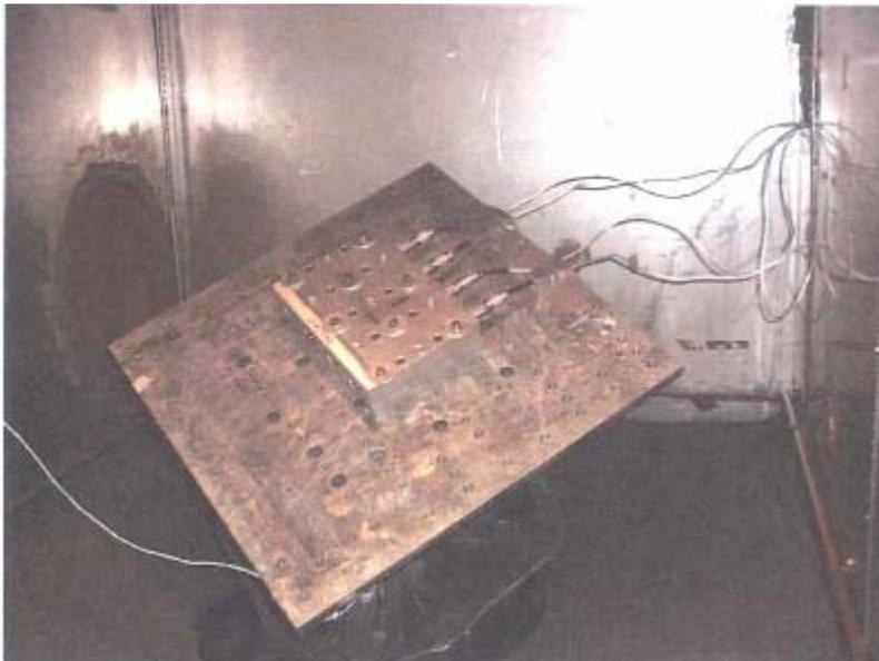
Figure 7. HALT Setup - Random Vibration on Skewed Fixture in Large Thermal Chamber.
