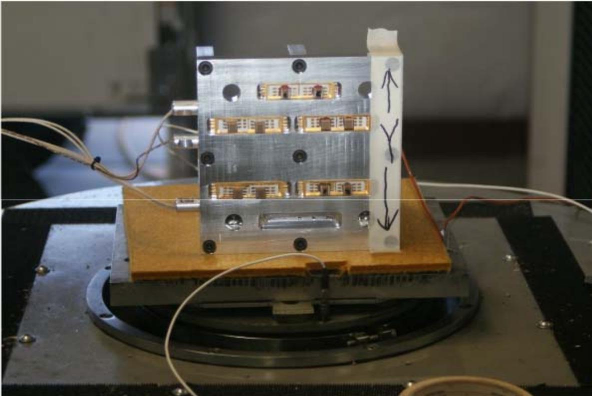
Figure 4. Hybrid Large Component Attach Heated Random Vibe Test
