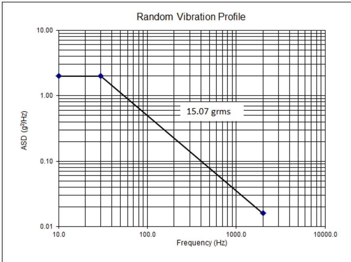
Figure 1. Typical 2000 Hz Random Vibration Profile
