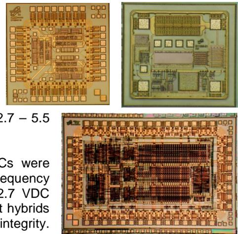
**Figure 6. Oscillator, Voltage Regulator and Frequency Counting ASICs improved circuit and sensor reliability.**
