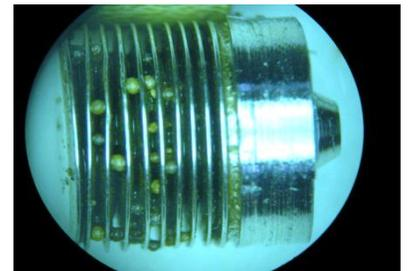
**Figure 10. Bellows damage caused by particulates trapped between convolutions.**
