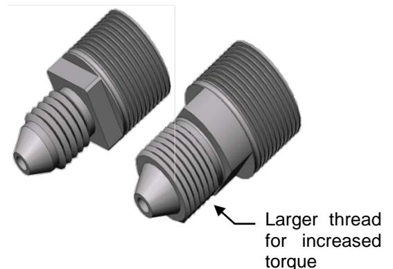
**Figure 9. Thread change provided increased reliability for bellows.**
