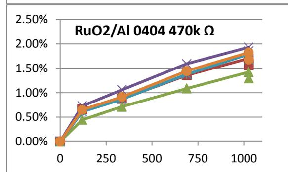
**Figure 5. Thick-film RuO<sub>2</sub> resistor aging. These particular units performed well, but are not typical of other resistors from the same family.**
