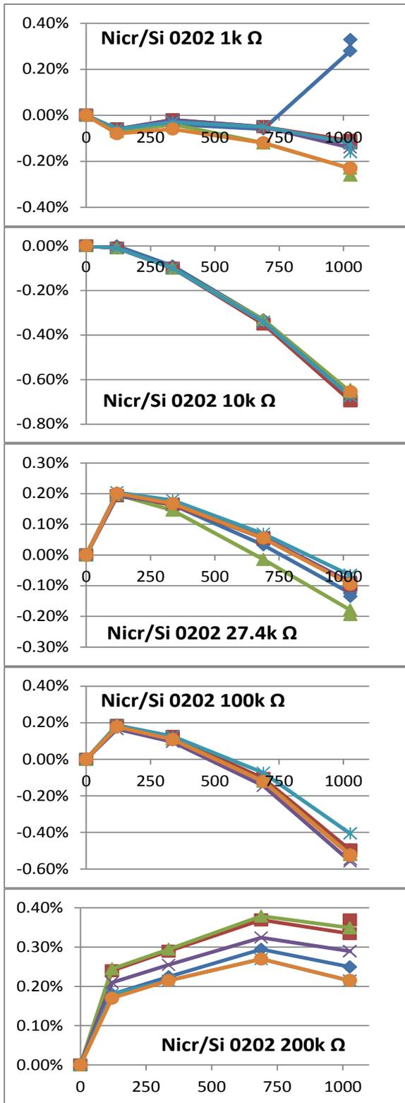
**Figure 8.** NiCr/Si resistors showing excellent aging performance over 1000 hours at 285°C: The outlying point on the 1k  $\Omega$  resistor is repeatable.
