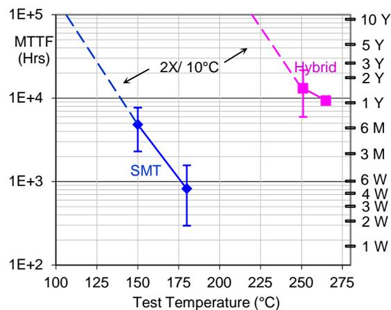
**Figure 1. Mean survival rates in non-powered Life-Cycle test. Error bars at 10 and 90%. Graph includes Surface-mount (SMT) and Hybrid data from 2003 thru Mar 2011.**
