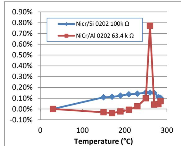
**Figure 11. Resistance change over temperature: The 260°C point for the 63.4k Ω resistor is likely in error. The probe was adjusted prior to the reading at 170°C.**
