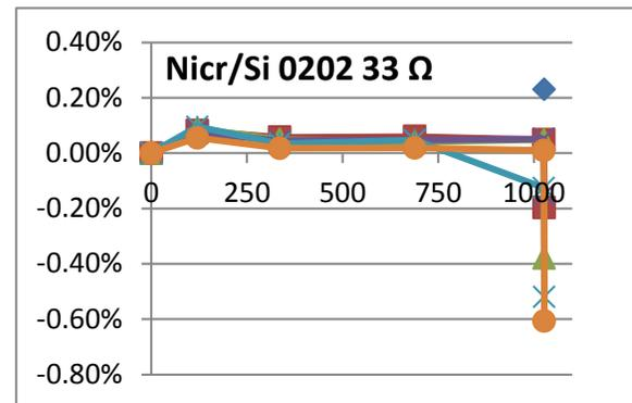
**Figure 7. 33 Ω NiCr/Si resistor showing good stability over time at 285°C, but a significant difference between through-wire bond and direct-on-die impedance after 1000 hours.**
