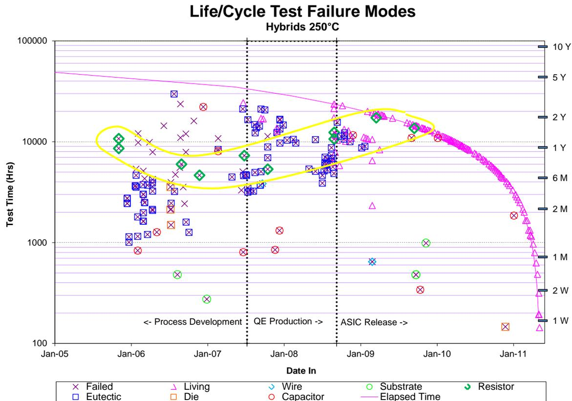
**Figure 2: 250°C Life-Cycle test failures. Each symbol represents a circuit in the test. Surviving units generally follow the elapsed-time curve. Failed units are marked with an “X” and a failure mode. Early Eutectic and Substrate failures were from parts built while we were developing our in-house process. Eutectic was removed from the process in 2008 with the introduction of the ASIC models. Resistor Drift is now the dominant wear-out mechanism. Capacitors are also becoming a concern.**
