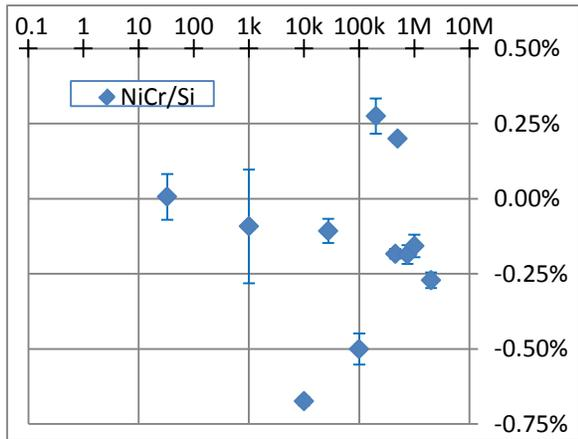
**Figure 12. Drift after 1000 hours at 285°C with error bars at +/-1 standard deviation: NiCr/Si is plotted separately on the second chart with a tighter vertical scale.**
