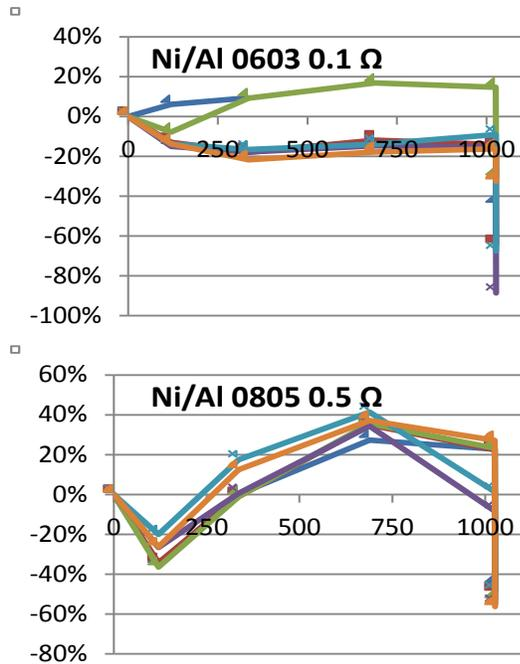
**Figure 10. Nickel alloy current-sense resistors: Aging is erratic with significant contribution from wire bond impedance.**
