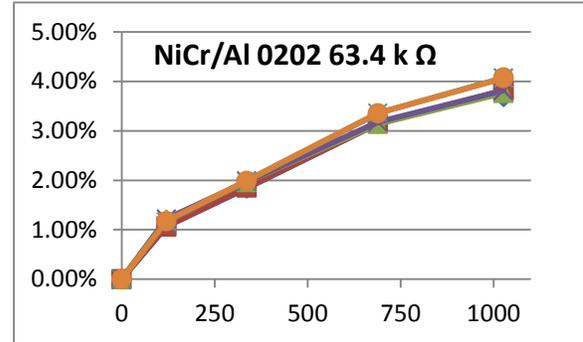
**Figure 4. NiCr/Al 63.4kΩ: The smooth exponential aging characteristic is typical of similar units in prior test. Individual units track each other well.**
