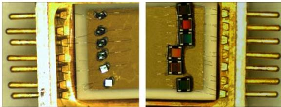
**Figure 3. Resistors placed in ends of hybrid package with contacts bonded to I/O pins for testing. Resistors share a common ground pin.**
