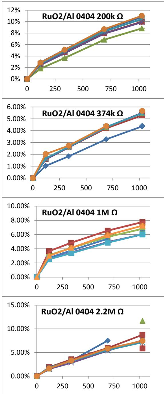
**Figure 6. Thick-film RuO<sub>2</sub> resistor aging: Drift ranging from 5-12% is higher than we would like to see, but may be acceptable for non-critical applications.**
