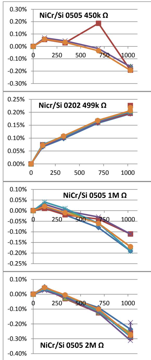
**Figure 9.** NiCr/Si resistors showing excellent aging performance over 1000 hours at 285°C: The outlying point on the 450k $\Omega$  resistor is likely a measurement error. No significant difference is observed when comparing package sizes (0202 vs. 0505).
