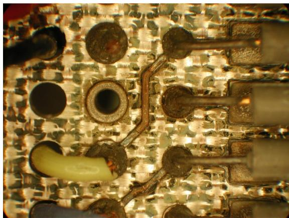
**Figure 6: Polyimide Thru-hole PCB after extended exposure to 225°C. The polyimide resin has mostly evaporated leaving a fragile mesh of fiberglass and copper.**
