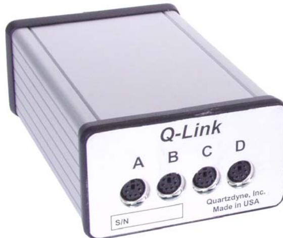
The serial computer interface allows the user to select the units of pressure and temperature, and permits zero and span adjustments. The user can select which data is transmitted to the computer. Q-Link automatically downloads any connected digital transducer's coefficient file. User-selected options (such as units of pressure and temperature) can be written to memory, so that the Q-Link operates in the desired mode on "power-up."
