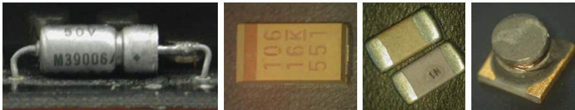
Figure 6. Capacitors (left to right): (a) wet-slug tantalum, (b) dry tantalum, (c) multilayer ceramic (NPO, X7R), and (d) ferrite bobbin inductor.
