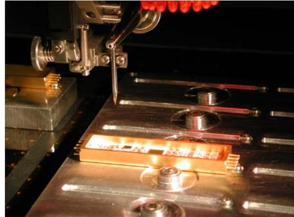
Figure 2. Automated Wire Bonder with Hybrid Circuit on heated parts stage: up to 12 parts can be loaded simultaneously.
