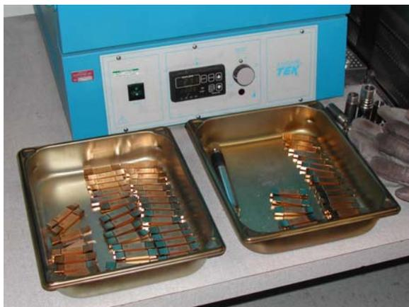
Figure 4. Hybrid Circuits in Life/Cycle test being cycled from 225°C to ambient temperature.
