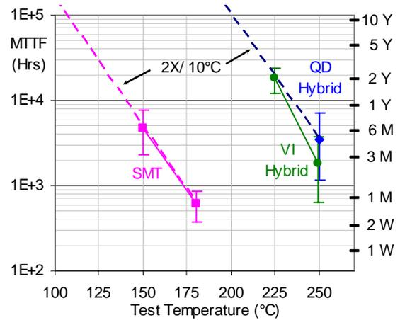
**Figure 8. Time to 50% failure for various circuit technologies in Life/Cycle test since July 2001 (error bars at 10% and 90%). Nominal de-rating of 2X/10°C is shown for reference.**
