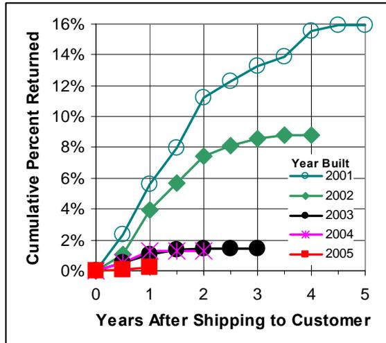
Figure 9. Cumulative customer return rate for Hybrid circuits. Each line represents the number units shipped in a given year that were returned for Hybrid circuit failure. The x-axis represents the number of years the unit was in the field before it was returned. The last two points of each series may still rise as the periods are not yet closed.
