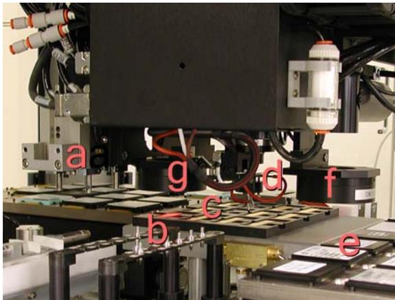
Figure 1. Automated Component Placement System: (a) polyimide dispense, (b) die collet holders, (c) substrates in placement area, (d) eutectic processing stage, (e) components in removable trays of waffle packs, (f) large area imaging camera, and (g) high resolution imaging camera.
