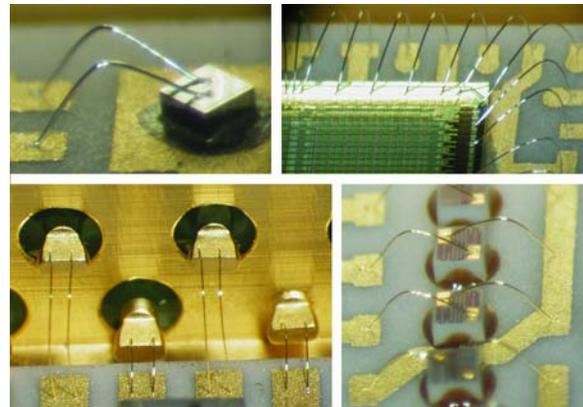
Figure 3. Wire bond samples: Al wires on a small transistor (top left) and a high-density FPGA (top right); Au bonds on staggered I/O pins (bottom left) and thin-film resistors (bottom right).
