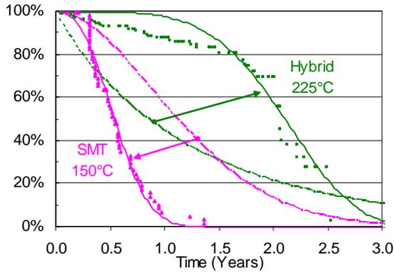
**Figure 7. Survival Rate plotted at each failure time for circuits built after 7/1/2001 (Dots). Solid lines are best-fit Weibull Survival Function for the same. Dashed lines are best-fit survival functions for circuits built prior to 7/1/2001.**
