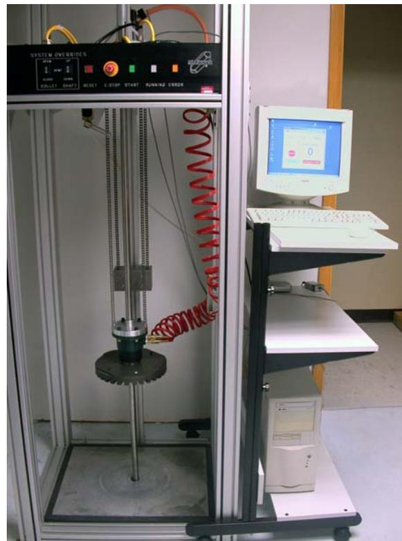
Figure 5. High-impact Drop Fixture. Under computer control, a pneumatic collet lifts the parts carrier to a pre-determined height and then releases it. A sleeve bearing keeps the carrier level during the fall.
