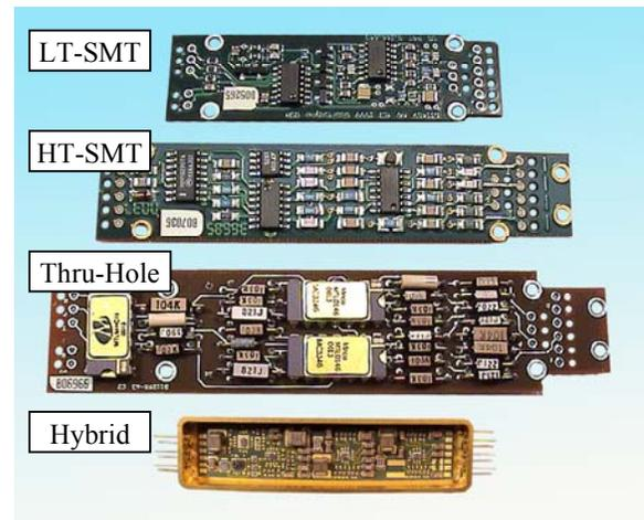
Figure 1. Photograph of boards typical of test units.
