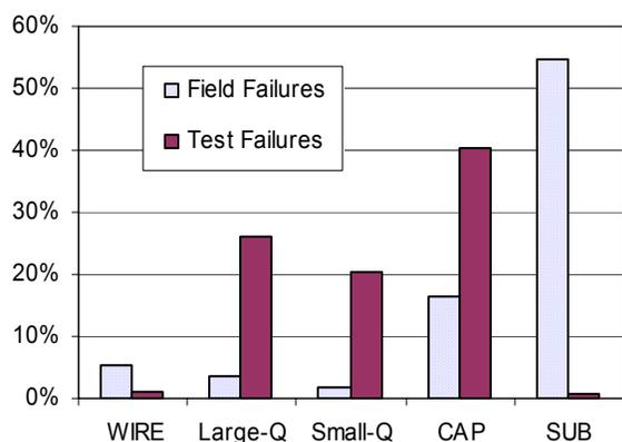
**Figure 8. Comparison of Field Failures to Life/Cycle Test Failures. While substrate detachment (SUB) is the most prominent field failure, it has been observed only once in Life/Cycle testing. Other failure modes show better correlation.**
