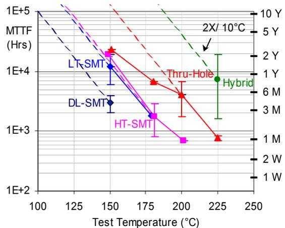
**Figure 4. Mean Time to Failure (MTTF) for various circuit technologies in Life/Cycle test. Error Bars at 10% and 90%. Nominal de-rating of  $2X/10^\circ\text{C}$  is shown for reference. The non-linearity of the Thru-Hole points suggests multiple independent failure mechanisms.**
