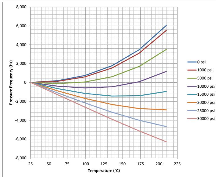
Figure 2. 30 kpsi pressure crystal temperature curves at various pressures. Linearity increases with pressure.
