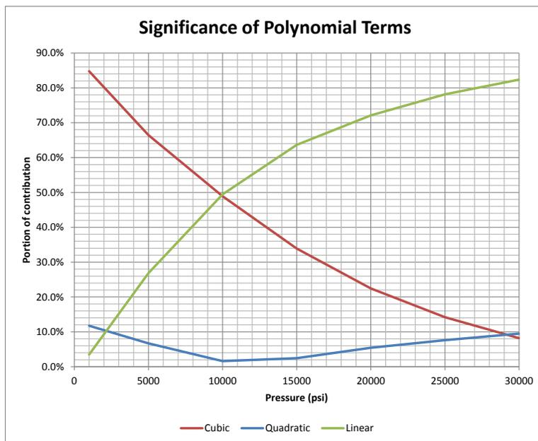
Figure 3. Significance of polynomial terms for pressure crystal curve fit. The cubic term is much stronger than the linear term at low pressure supporting the observed curvature in Figure 2.
