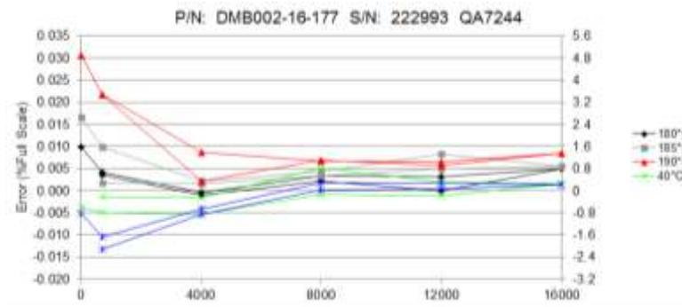
Figure 1. QA loops of DMB002-16-177 transducer. Three additional loops are added to test extrapolation. Performance at low pressure is clearly diminished.
