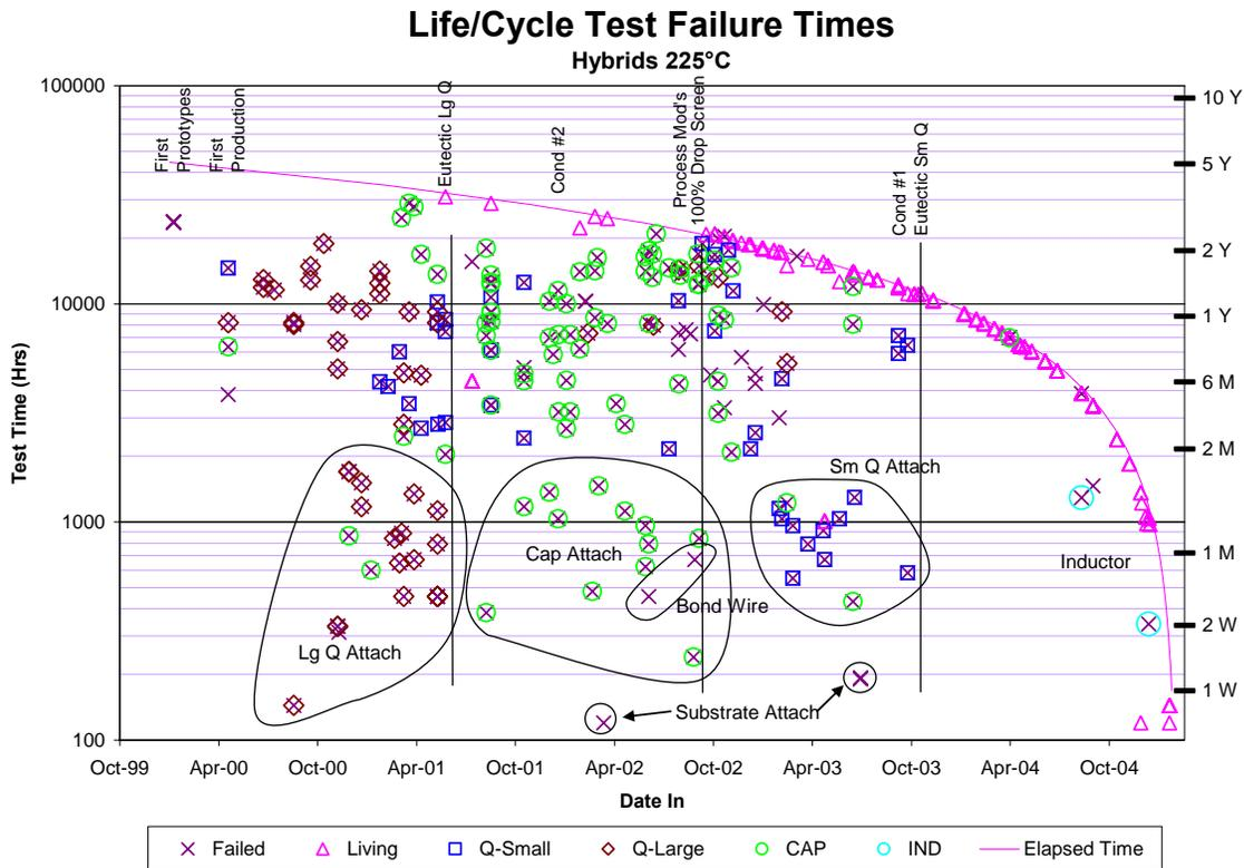
**Figure 4. Test times for production hybrid units in Life/Cycle test. Failed units are denoted with an "X"; open triangles "△" indicate units still surviving. The latter generally follow the elapsed time line until failure. Failure modes and key process changes are also identified.**
