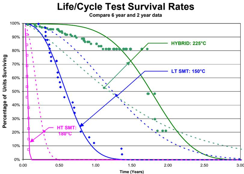
Figure 3. Survival Rate plotted at each failure time for the last 2 years only (July 2003 through July 2005). Solid lines are best-fit Weibull survival function for 2 year data. Dashed lines are from 6 year data. Note the improvement in Hybrids, while the SMT technologies have become worse.
