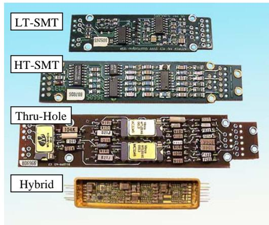
**Figure 1. Oscillator Circuits Tested**
