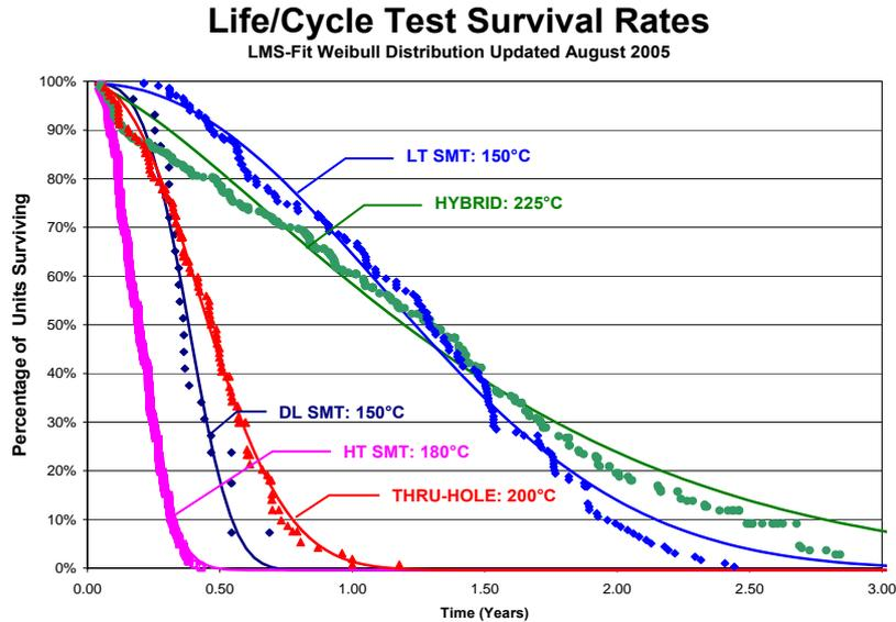
Figure 2. Survival Rate plotted at each failure time for primary test temperatures. Smooth lines are best-fit Weibull Survival Function based on testing from April 1998 through July 2005.
