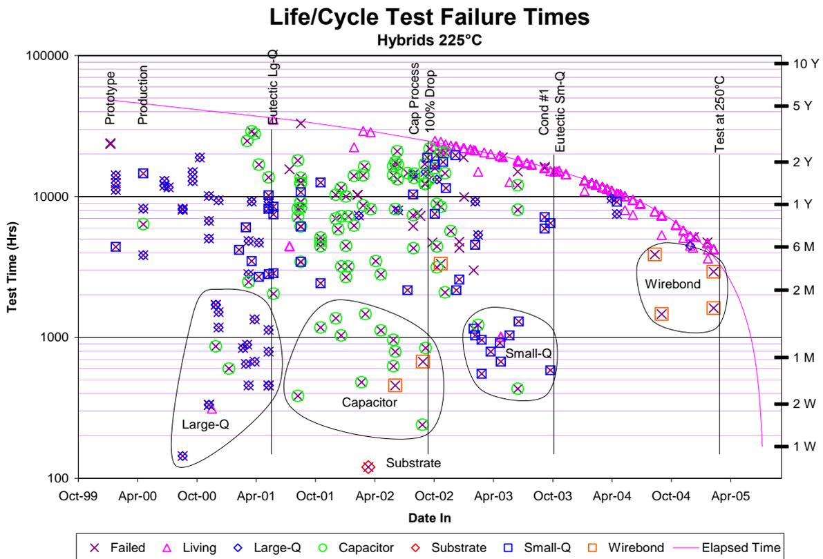
**Figure 4. Test times for production hybrid units in Life/Cycle test at 225°C. Failed units are denoted with an "X"; open triangles "Δ" indicate units still surviving. The latter generally follow the elapsed time line until failure. Failure modes and key process changes are also identified.**
