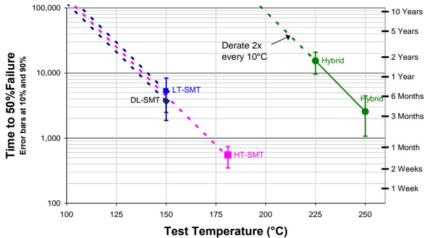
Figure 6. Life/Cycle test time to failure based on last 2 years of testing.
