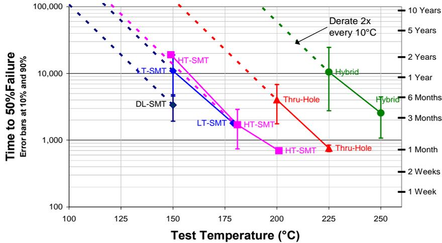
Figure 5. Life/Cycle test time to failure based on 6 years of testing.
