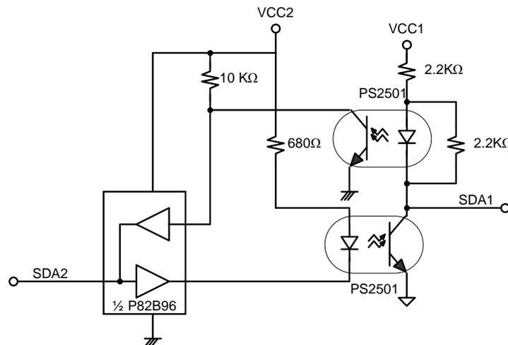
**Figure 3. Isolated I<sup>2</sup>C buffer. Circuit is repeated for SCL.**
