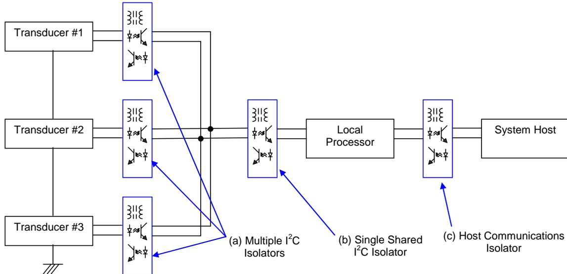
**Figure 4. Three options for electrical isolation within a system: (a) Multiple isolation units at or near each transducer, (b) a single isolation unit at the local host, shared by all transducers, or (c) a single isolation unit between the local processor and the system host.**
