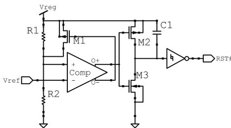
Figure 3 Microprocessor Reset
