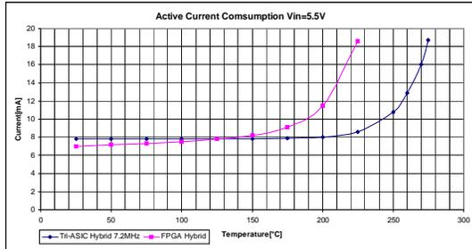
**Figure 14 FPGA vs ASIC Module Current**
