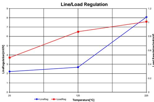
**Figure 8 Line and Load Regulation**
