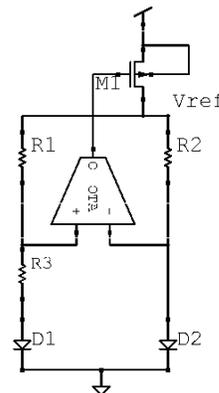
**Figure 2 BandGap Voltage Generator**
