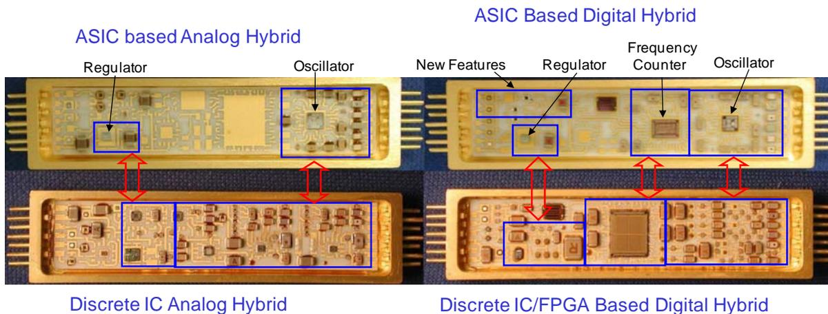
**Figure 15 Hybrid Circuit Comparisons**
