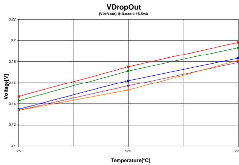
**Figure 7 Dropout Voltage**
